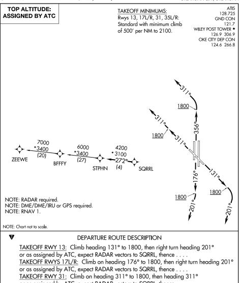
or as assigned by ATC, expect RADAR vectors to SQRRL, thence . . . . <u>TAKEOFF RWYS 35L/R:</u> Climb on heading 356° to 1800, then left turn heading 311° or as assigned by ATC, expect RADAR vectors to SQRRL, thence . . . .
